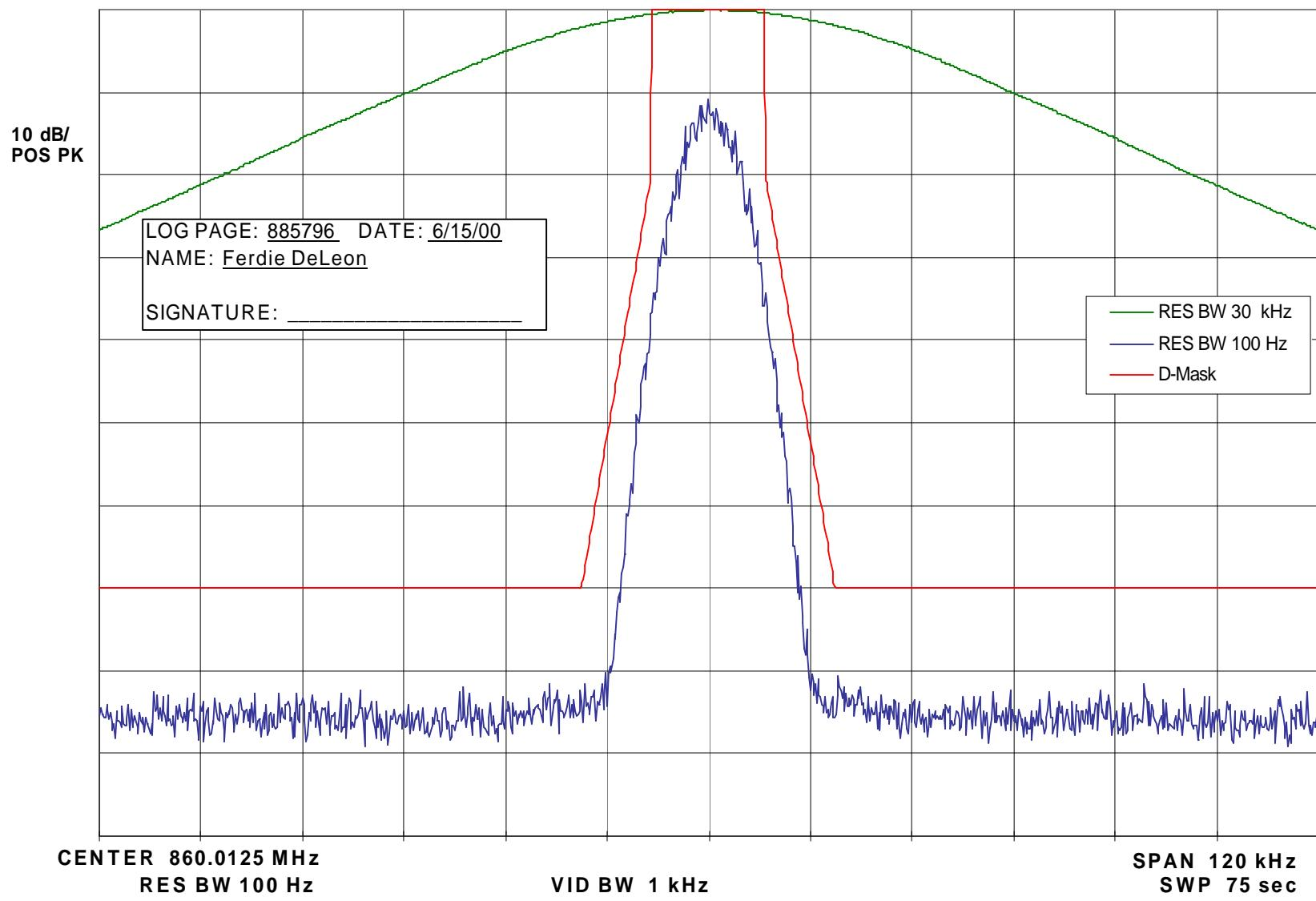
**CONDUCTED SPURIOUS EMISSIONS****SPECIFICATION REQUIREMENT:****Reference: Part 90.210 (Emission Mask D)**
