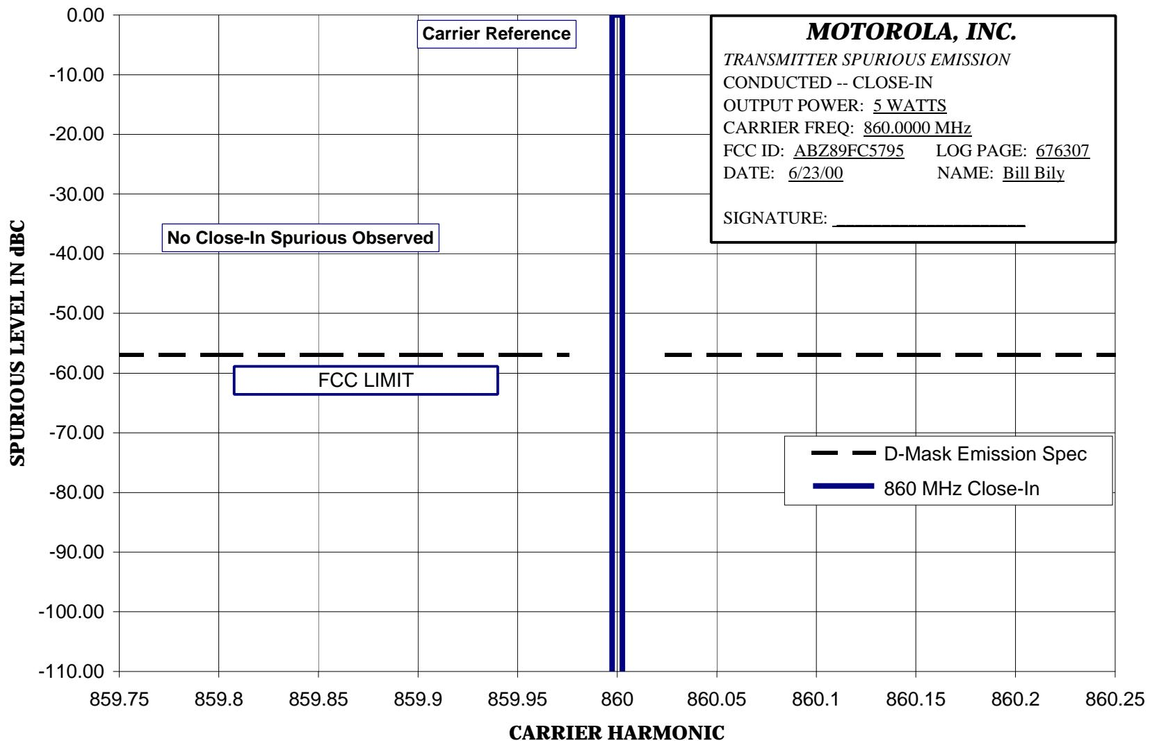
**RADIATED SPURIOUS EMISSIONS****SPECIFICATION REQUIREMENT:****Reference: Part 90.210 (Emission Mask D)**
