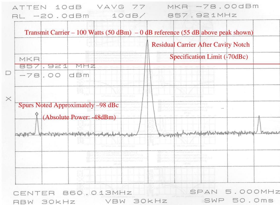
Note: The absolute power of the spurs were verified using the substitution method. The signal generator was fed into the same notch test setup as the transmitter. The power level of an 857.921 MHz signal was adjusted until equivalent power level as the spur shown above (-78dBm) was observed at the spectrum analyzer. This absolute power level was then compared to the power level of the transmitter to obtain the level of the spur referenced to carrier power.
