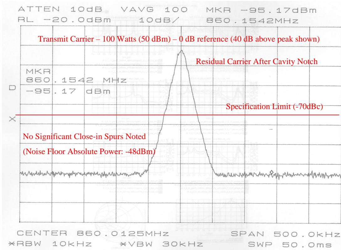
Note: The absolute power of spurious was verified using the substitution method. The signal generator was fed into the same notch test setup as the transmitter. The power level of an 860.1125 MHz (100 kHz offset from carrier) signal was adjusted until equivalent power level as the noise floor marker shown above (-95 dBm) was observed at the spectrum analyzer. This absolute power level was then compared to power level of the transmitter to obtain level of noise floor referenced to carrier power.
