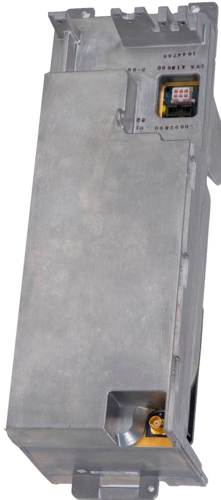
Internal Front View – Power Amplifier Module
