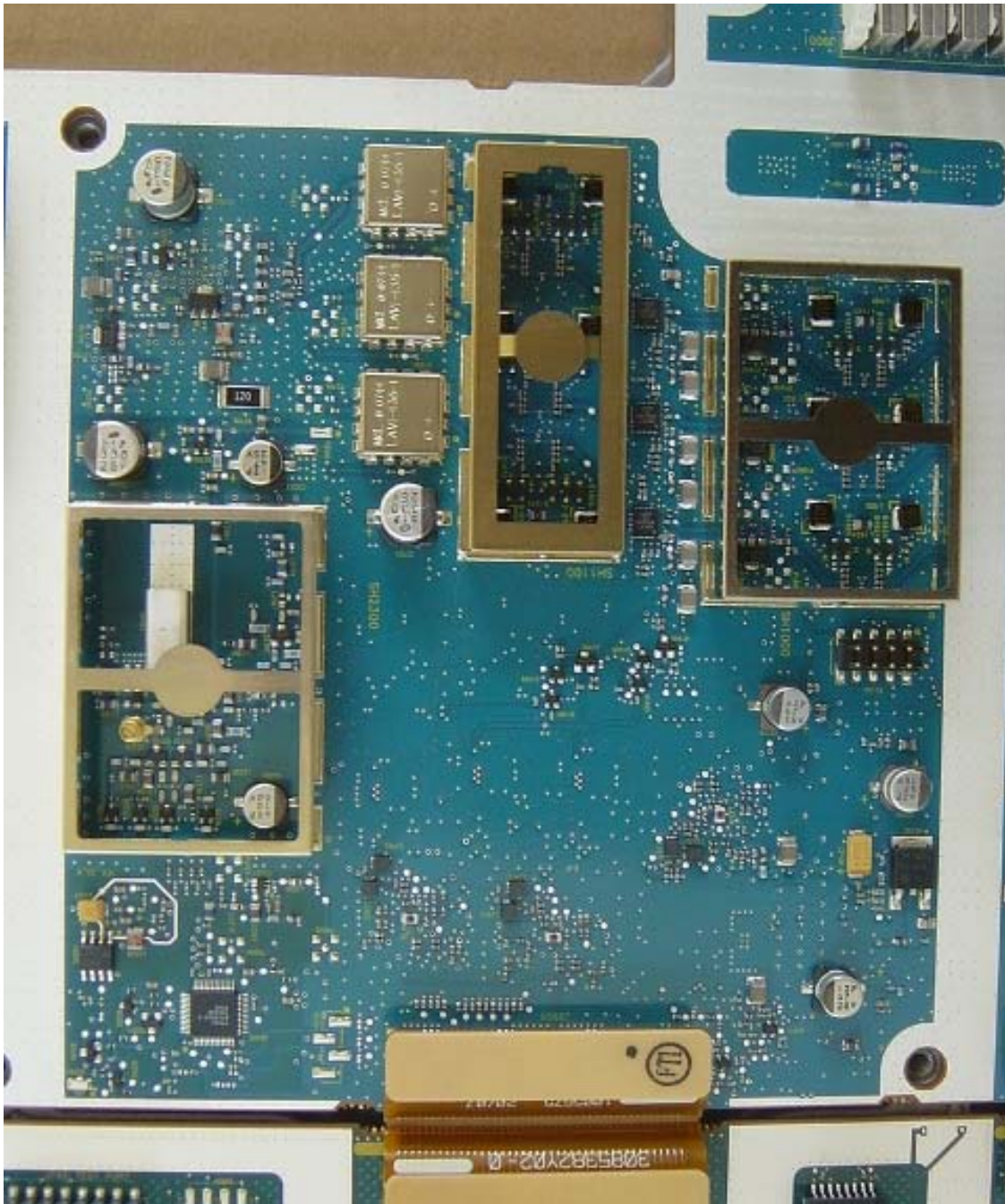
Internal Front View – Transceiver Module, Receiver Section
