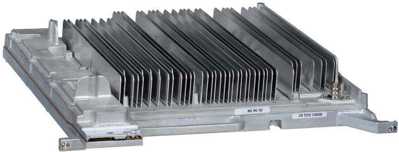
Internal Back View – Power Amplifier Module
