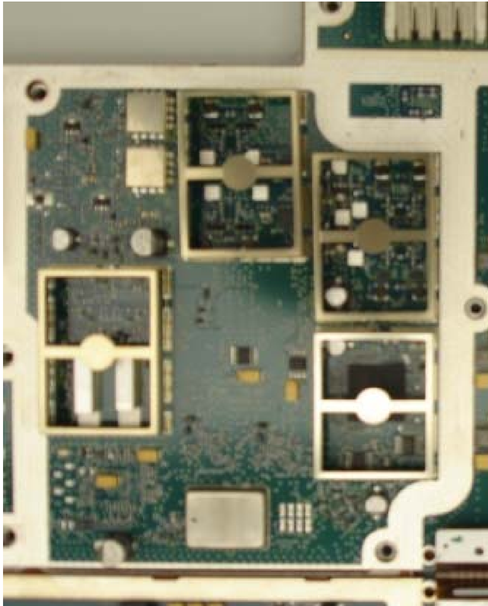
Internal Front View – Transceiver Module, Receiver Section
