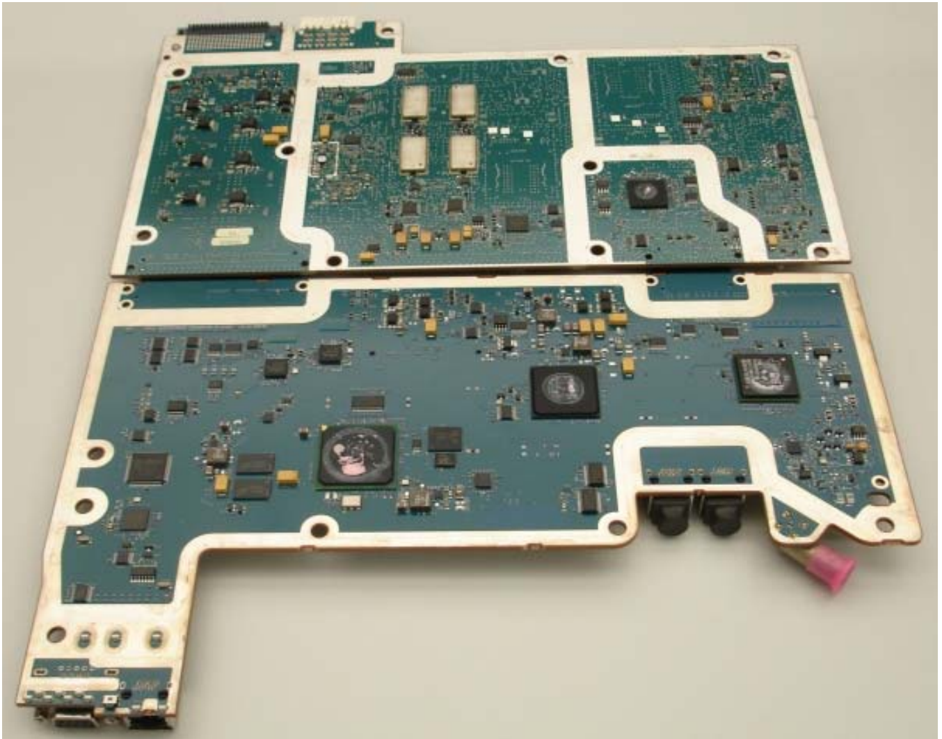
Internal Back View – Transceiver Module
