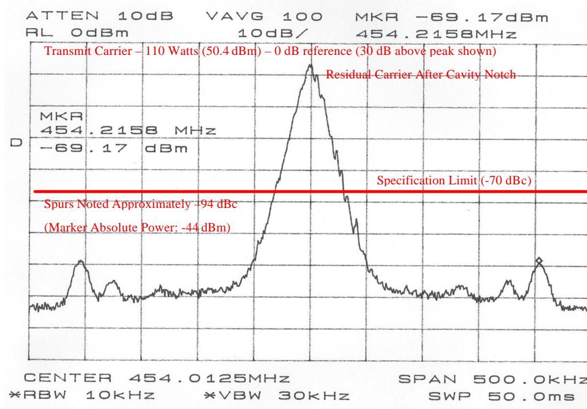
The absolute power of the spur was verified using the substitution method. A signal generator was fed into the same notch test setup as the transmitter. The power level of a 454.2158 MHz signal was adjusted until equivalent power level as the spur shown above (-69.17 dBm) was observed at the spectrum analyzer. This absolute power level was then compared to the power level of the transmitter to obtain the spur power level referenced to the carrier power.
