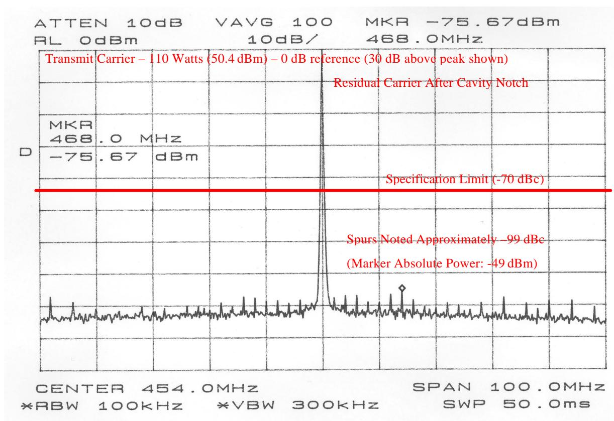
The absolute power of the spur was verified using the substitution method. A signal generator was fed into the same notch test setup as the transmitter. The power level of a 468.0 MHz signal was adjusted until equivalent power level as the spur shown above (-75.67 dBm) was observed at the spectrum analyzer. This absolute power level was then compared to the power level of the transmitter to obtain the spur power level referenced to the carrier power.
