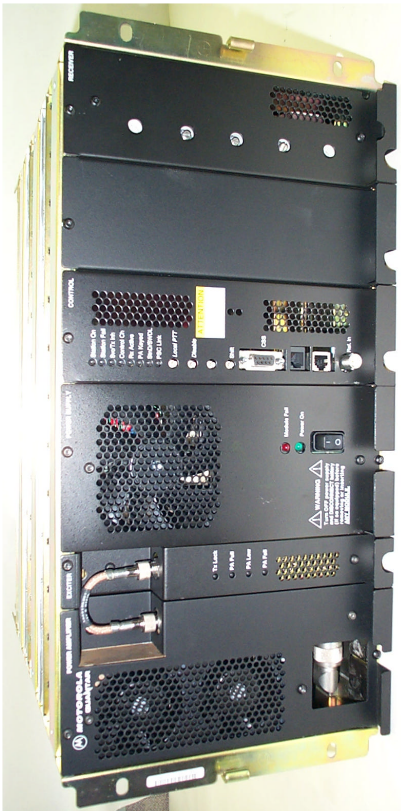
Base Radio -- Front View
