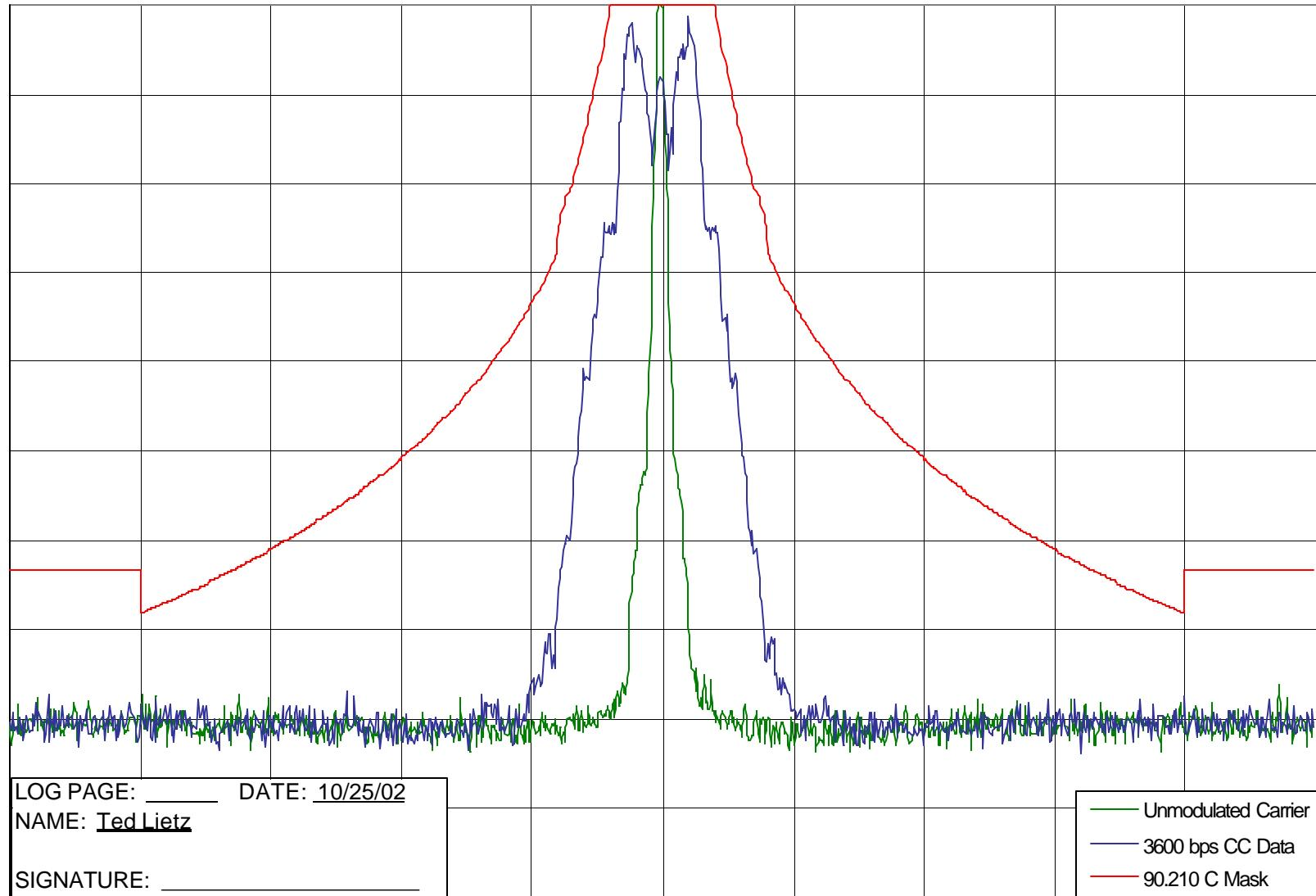
**CONDUCTED SPURIOUS EMISSIONS****SPECIFICATION REQUIREMENT:****§ 90.210(d) Emission Mask Requirements for 12.5 kHz Channel Bandwidth Equipment, Emission Mask D:**
