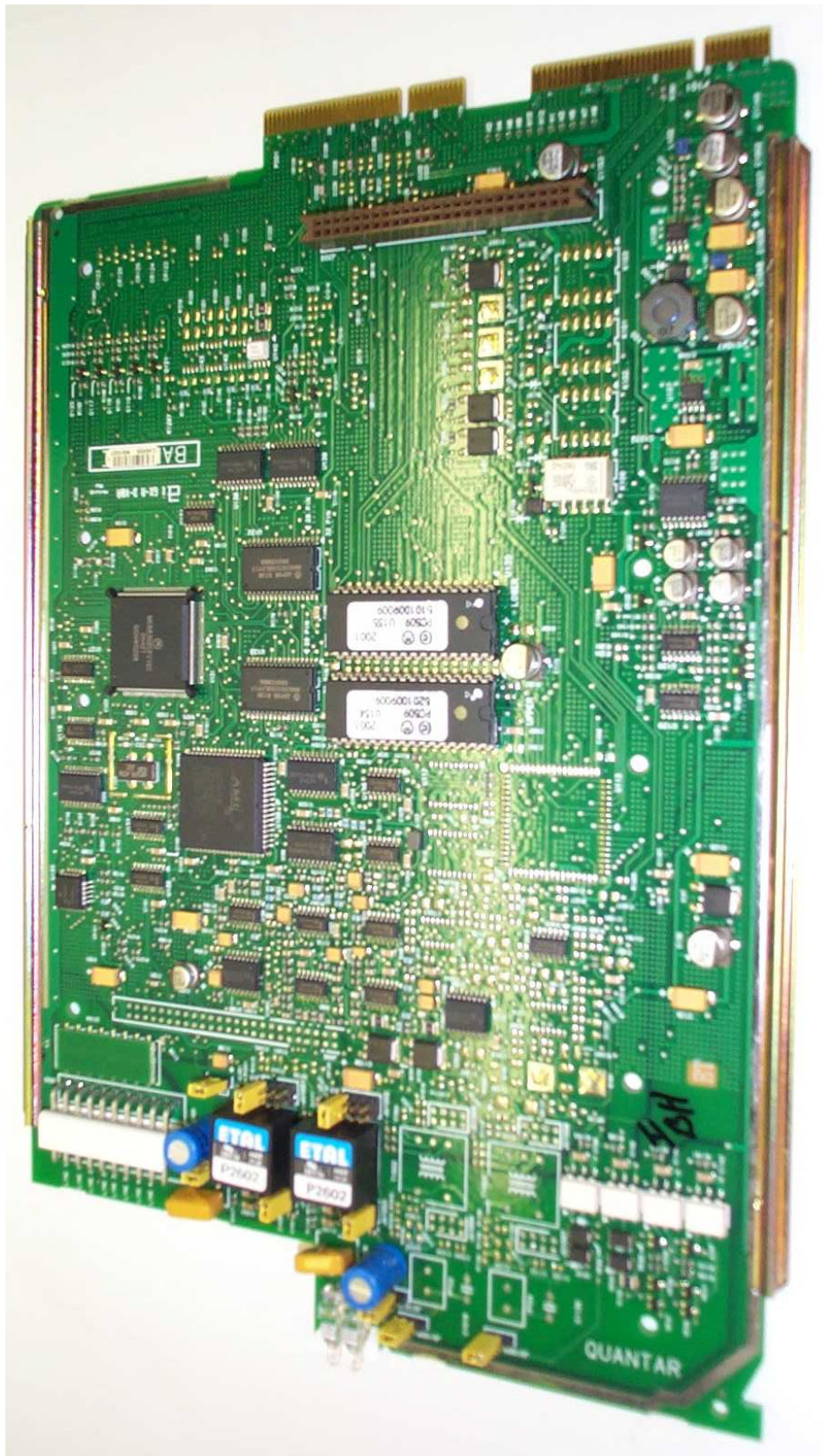
Wireline Module, Top Side
