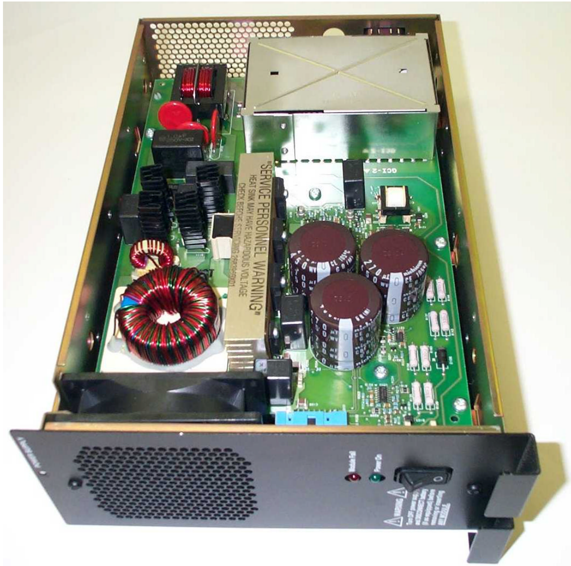
Power Supply Module, Cover Removed
