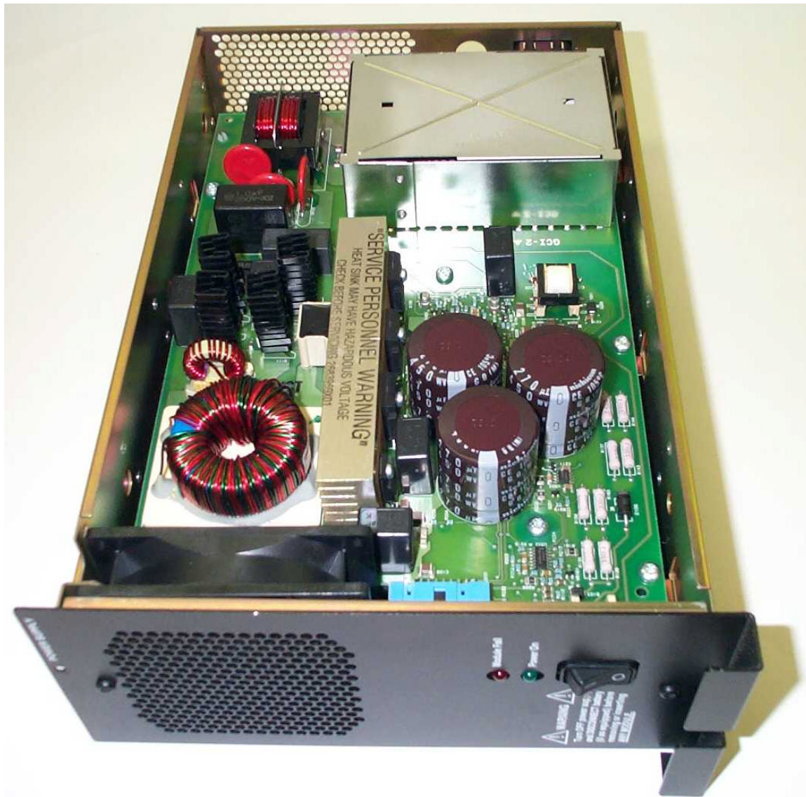
Power Supply Module, Cover Removed
