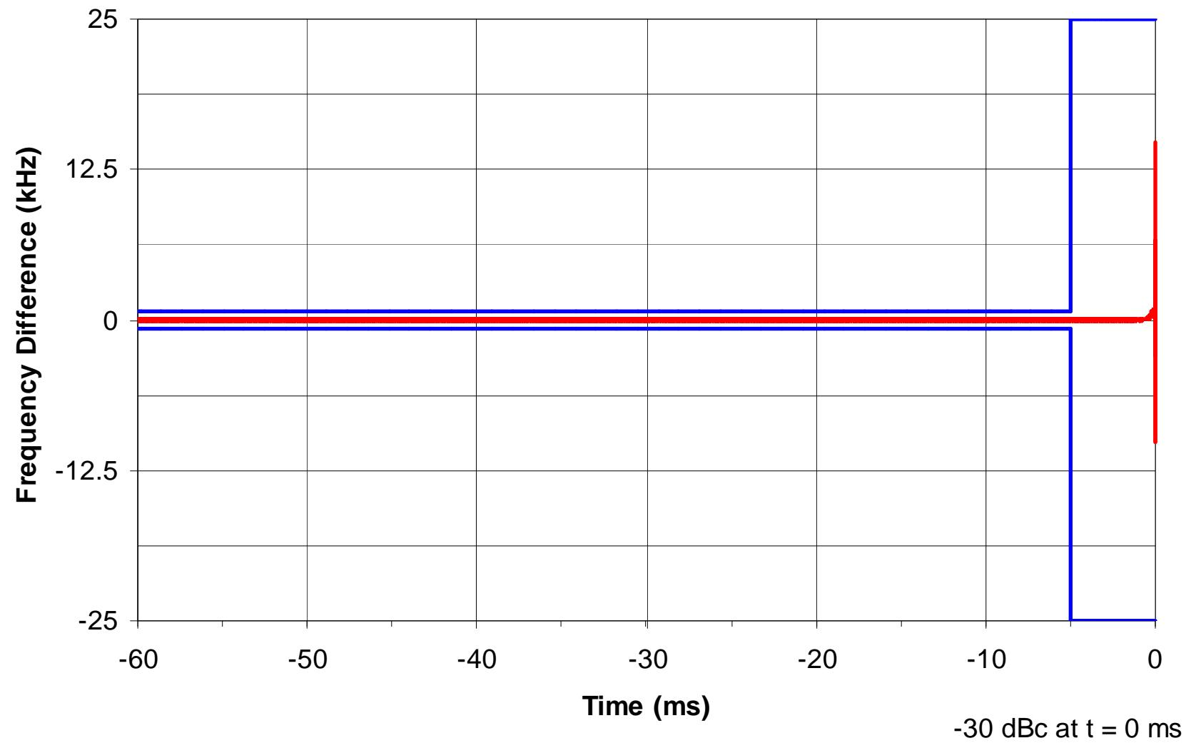
Frequency Transient – Key-up – 12.5 kHz Channels
