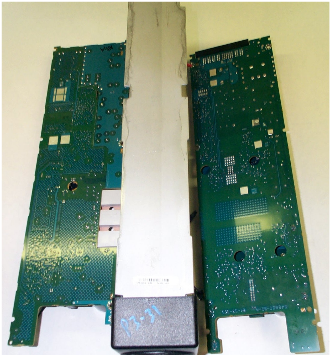
Internal Back View – Power Supply Module, Circuit Boards, Back View
