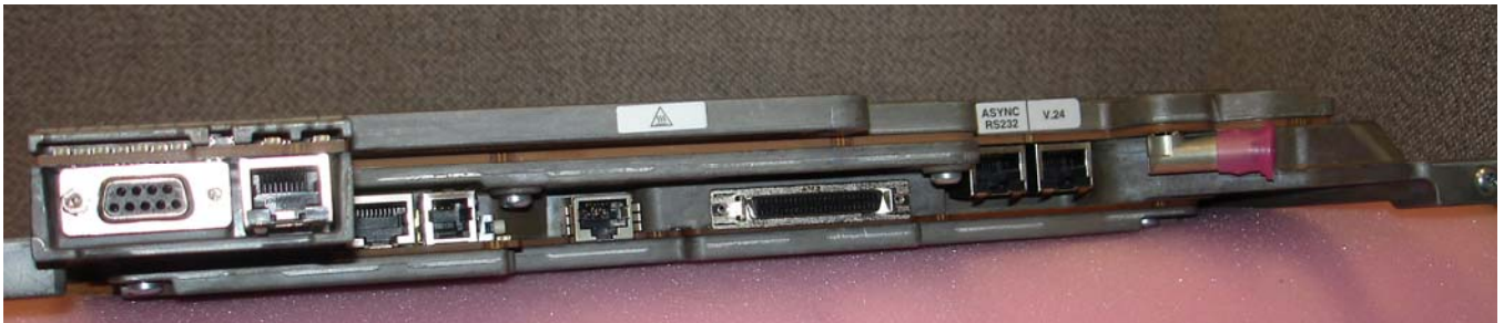
Transceiver Module with the Supplementary Audio Card (SAC) Installed
