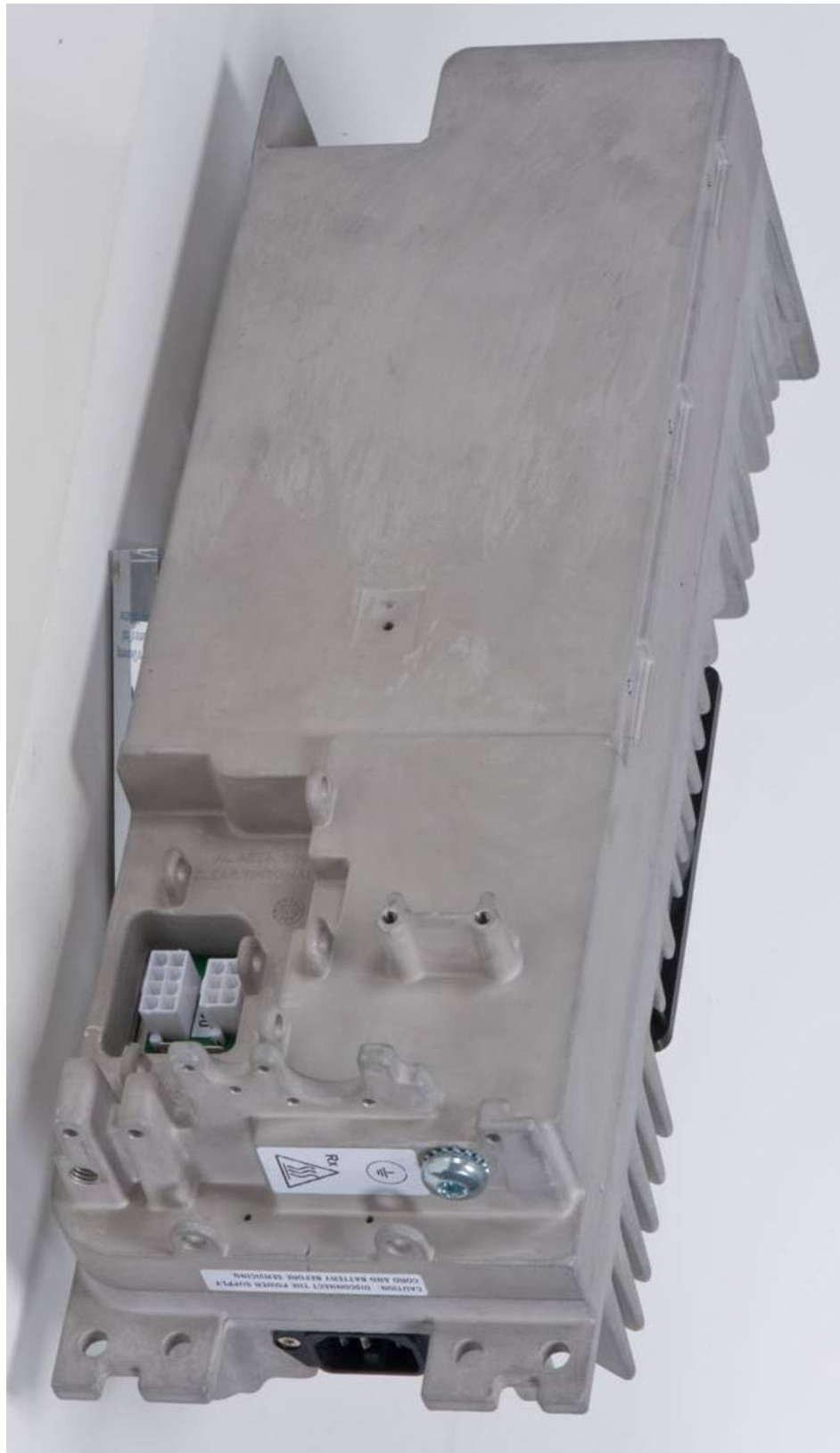
Internal Front View – Power Supply Module
