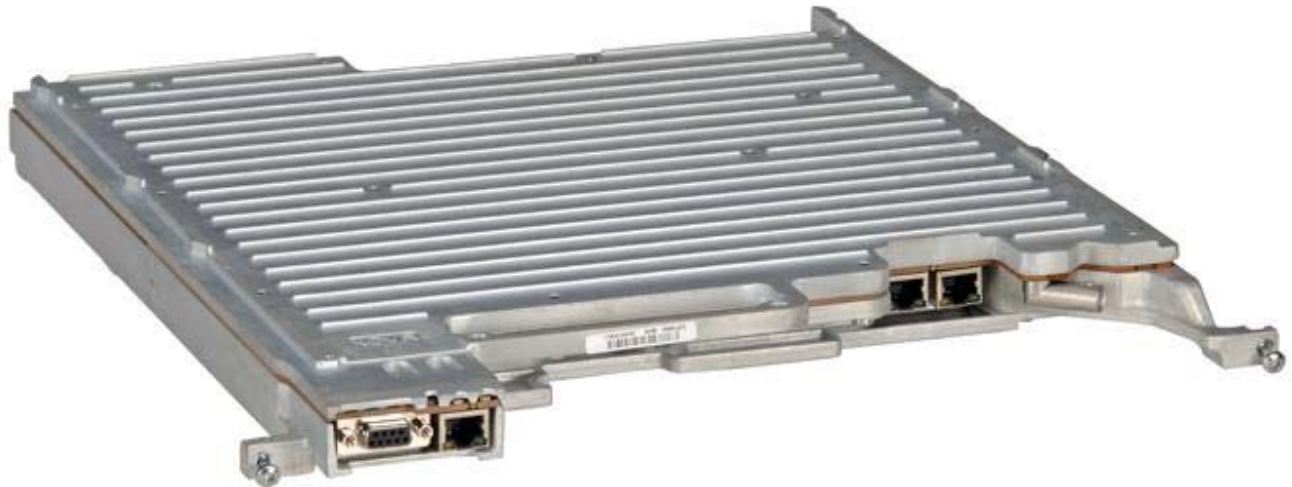
Transceiver Module without the Supplementary Audio Card (SAC)
