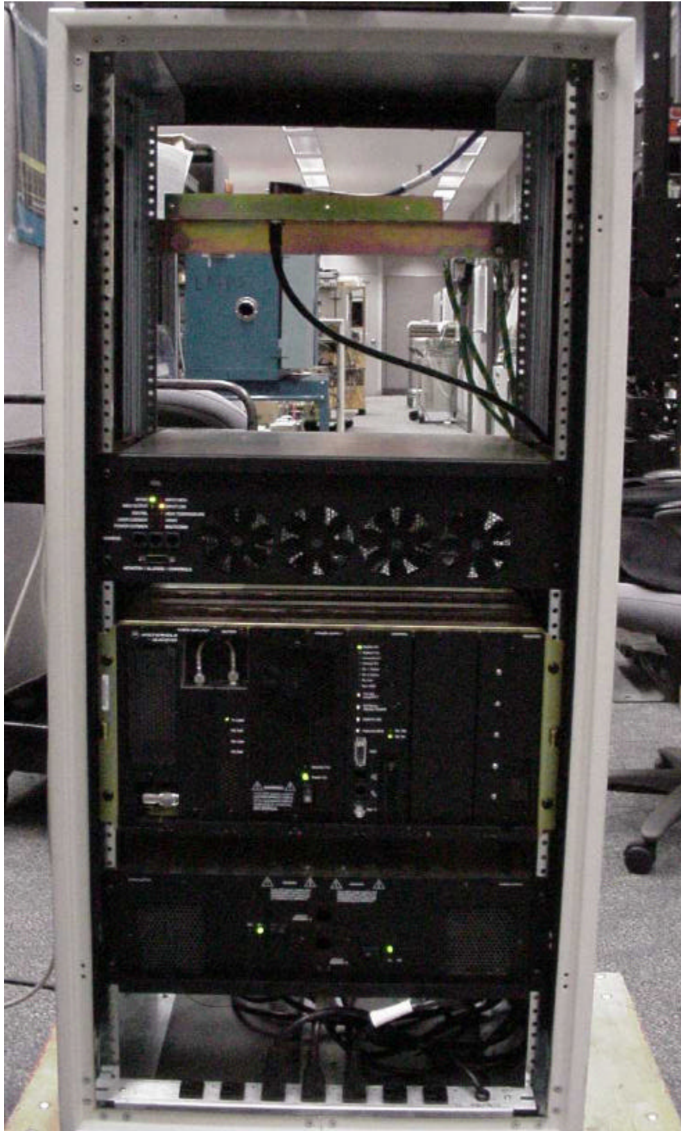
Rear View of Booster Amp Racked with Associated Base Station
