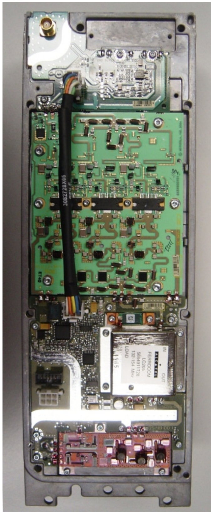
Power Amplifier Module, Front View, Cover Removed
