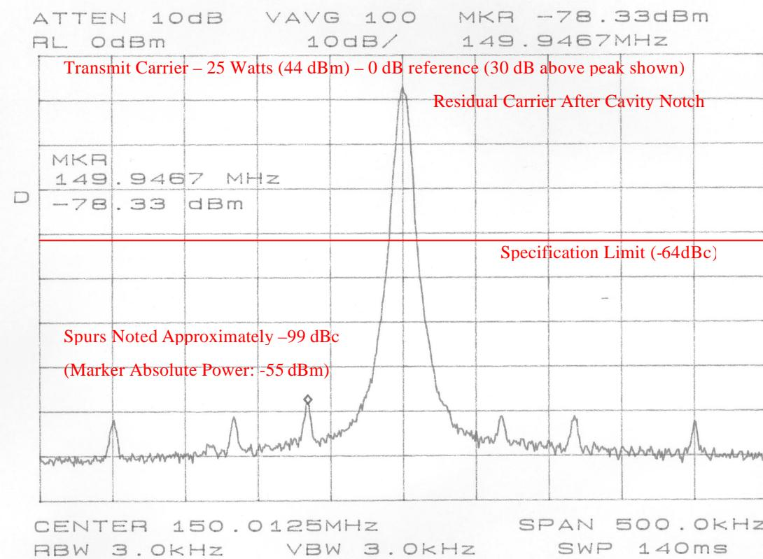
The absolute power of the spur was verified using the substitution method. A signal generator was fed into the same notch test setup as the transmitter. The power level of a 149.9467 MHz signal was adjusted until equivalent power level as the spur shown above (-78.33 dBm) was observed at the spectrum analyzer. This absolute power level was then compared to the power level of the transmitter to obtain the spur power level referenced to the carrier power.
