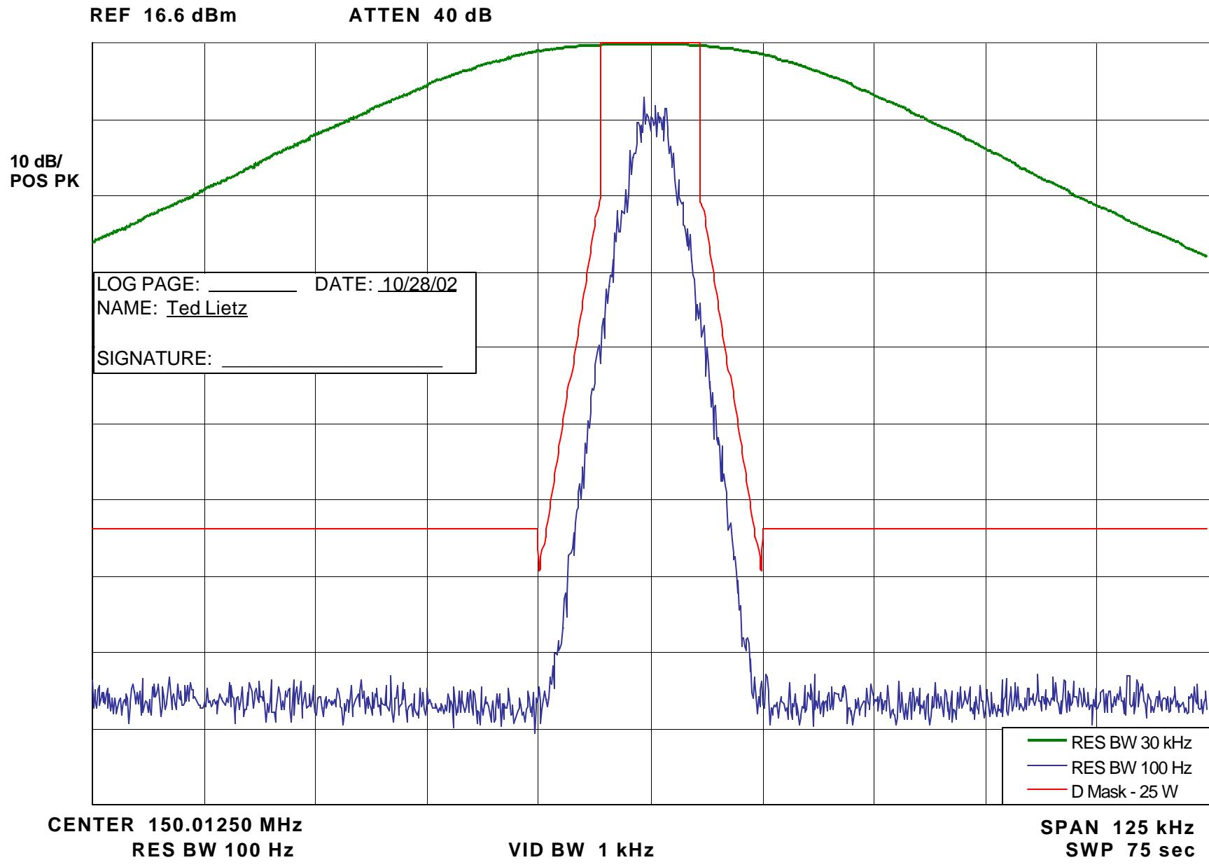
**CONDUCTED SPURIOUS EMISSIONS****SPECIFICATION REQUIREMENT:****§ 90.210(d) Emission Mask Requirements for 12.5 kHz Channel Bandwidth Equipment, Emission Mask D:**
