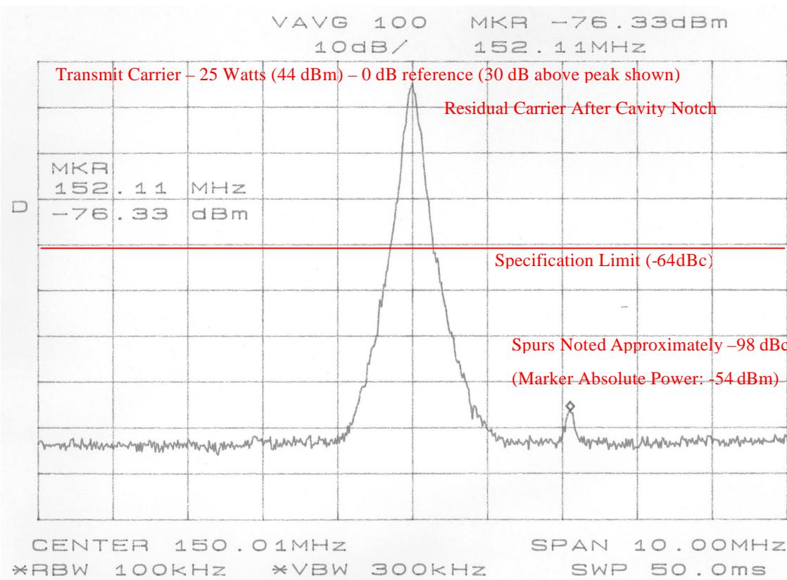
The absolute power of the spur was verified using the substitution method. A signal generator was fed into the same notch test setup as the transmitter. The power level of a 152.11 MHz signal was adjusted until equivalent power level as the spur shown above (-76.33 dBm) was observed at the spectrum analyzer. This absolute power level was then compared to the power level of the transmitter to obtain the spur power level referenced to the carrier power.
