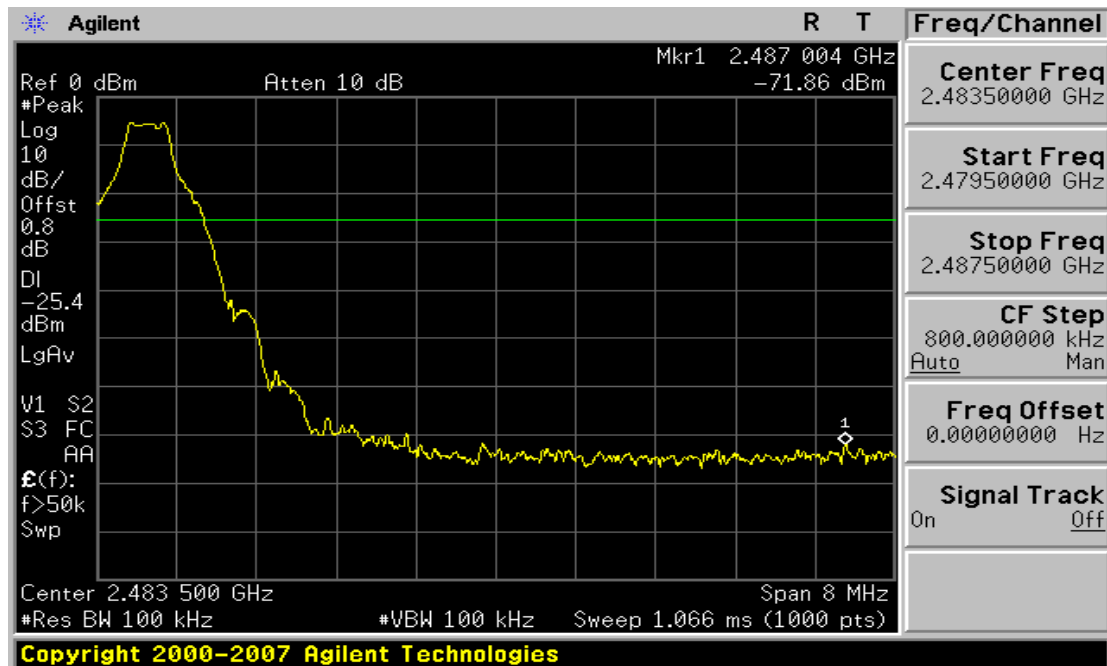
Plot 6-5. Band Edge Plot (Bluetooth – Ch. 78)
