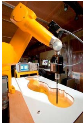
Figure 3-1 SAR Measurement System
