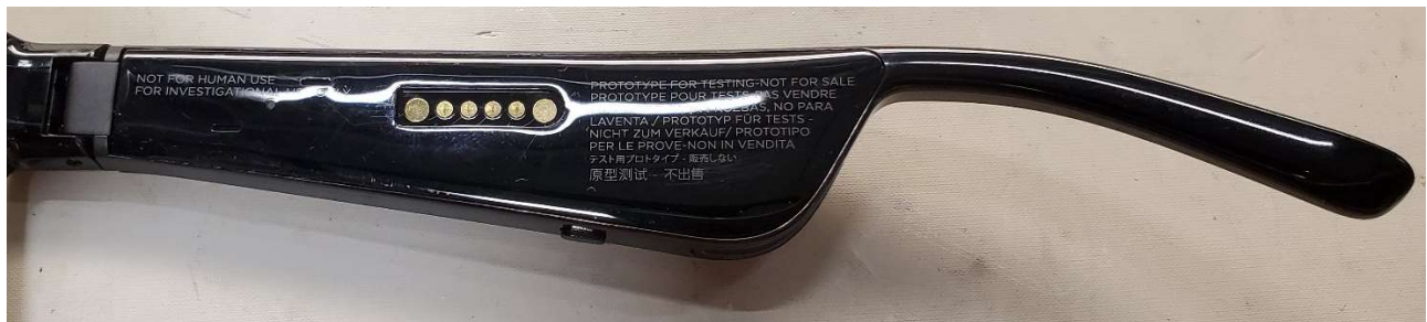
Right temple with charging cable connection, LED, and switch
