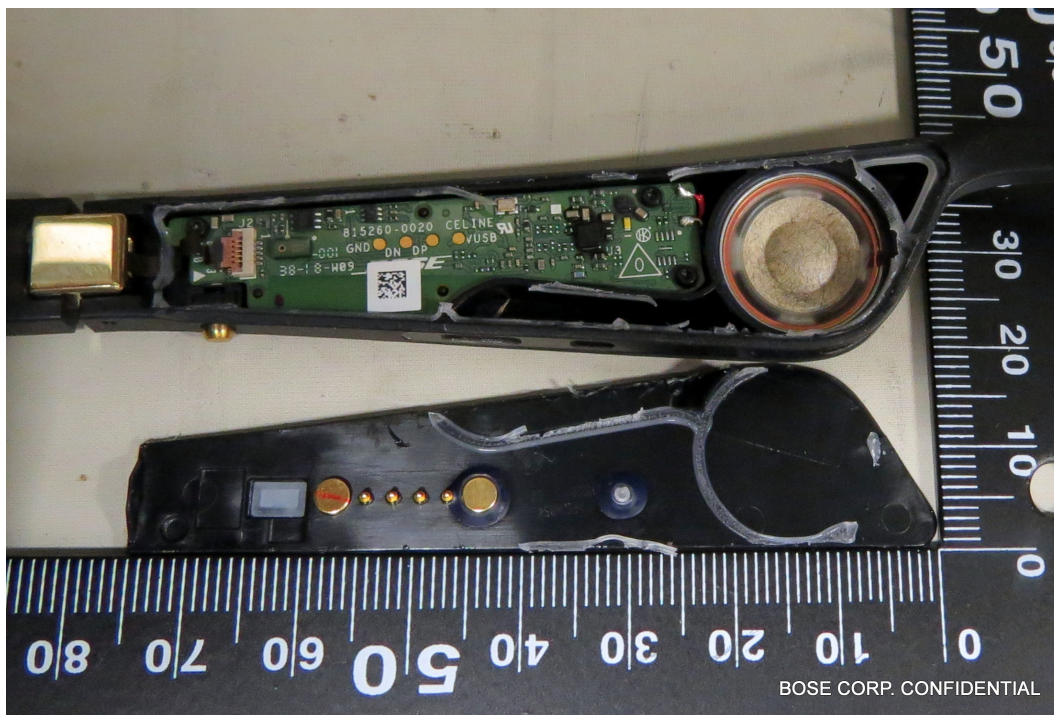
Charging Connector to main board connection, Right temple
