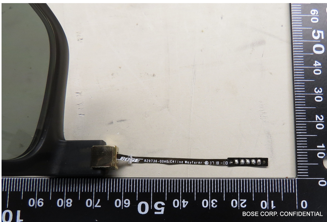
Left temple FFC connection (FFC is molded into the lens frame)
