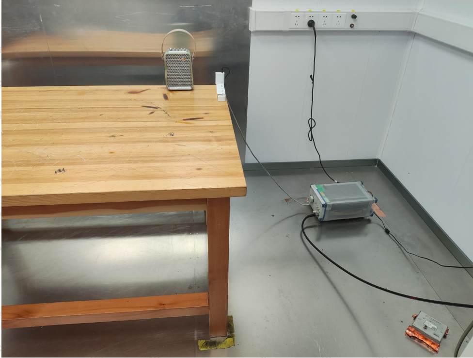
Photo of Radiation Emission Test (below 1GHz)
