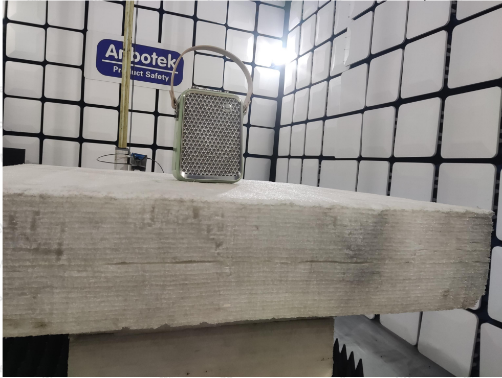
Photo of Radiation Emission Test (above 1GHz)
