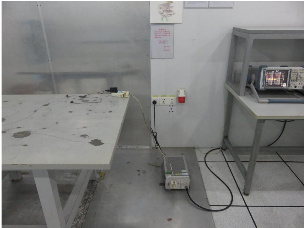
Photo of Conducted Emission Test
