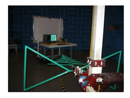
Figure 2 Radiated Emission Test Setup
