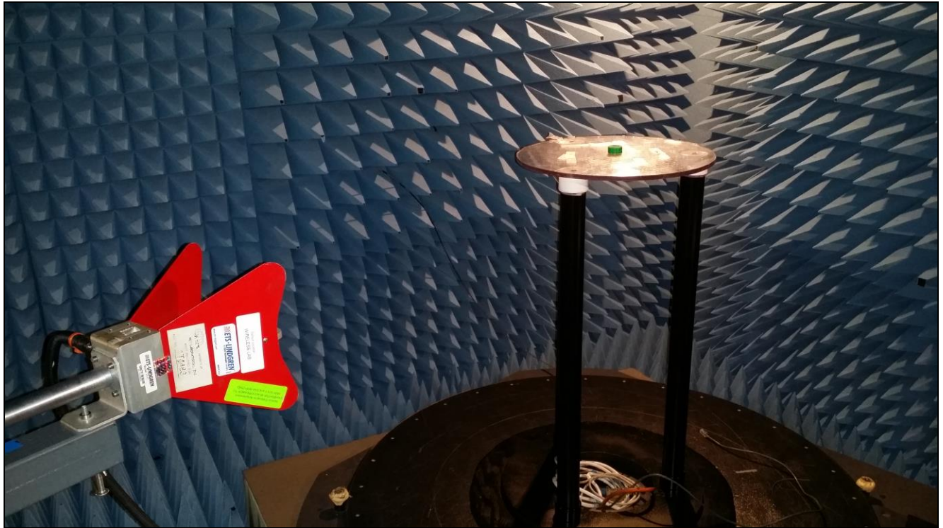
Photograph 1. Radiated Spurious Emissions, Test Setup
