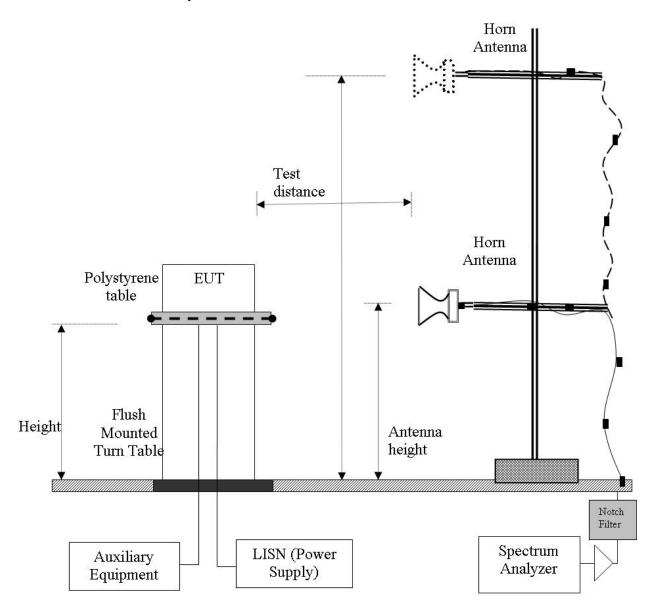
Radiated Emission Measurement Setup – Above 1 GHz
