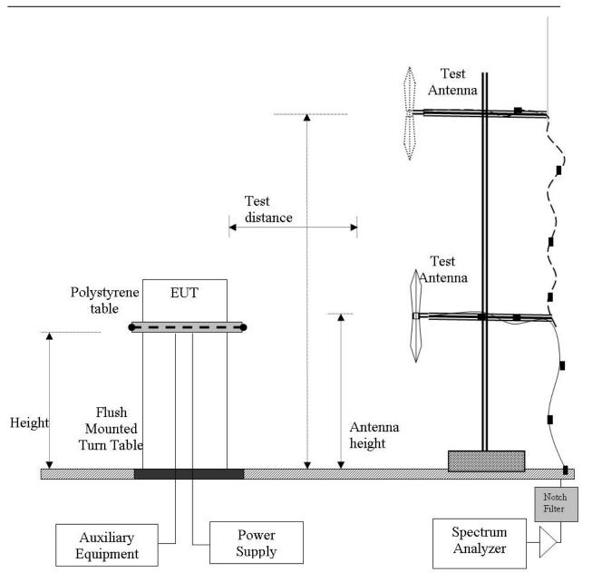
Radiated Emission Measurement Setup – Below 1 GHz
