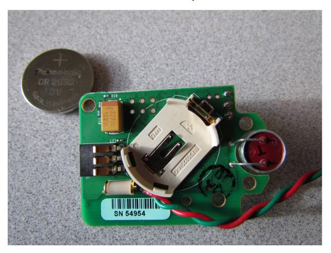
CP-500 with test leads to supply 3 Vdc power. CR2032 button battery to power under normal conditions
