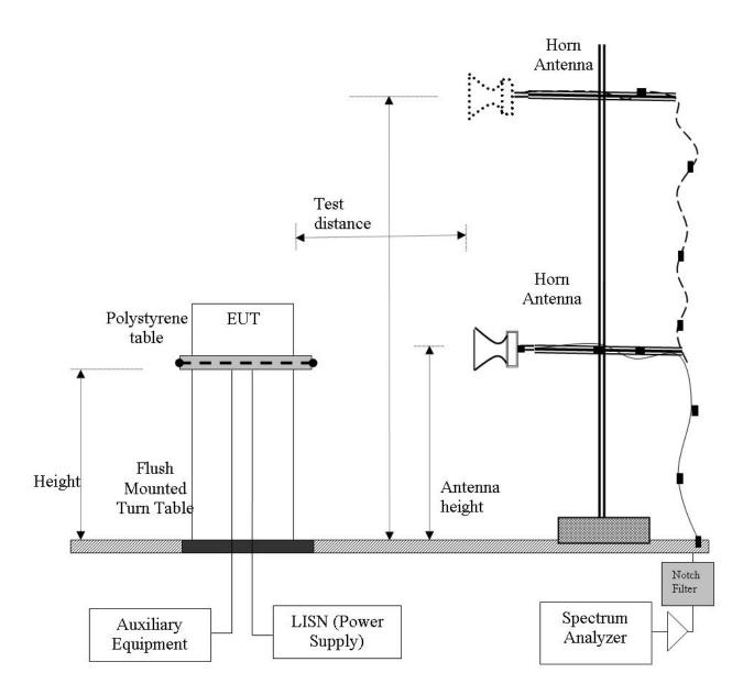
Radiated Emission Measurement Setup - Above 1 GHz
