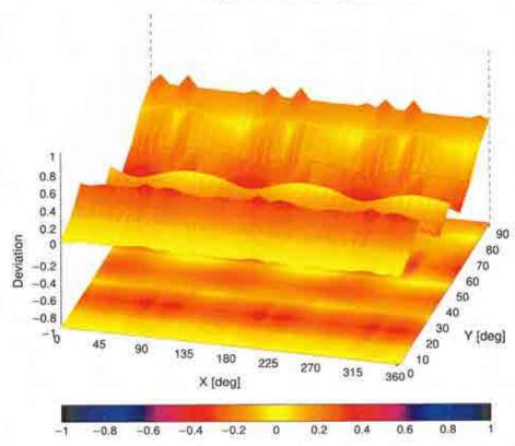
Probe isotropy for  $E_{tot}$ : probe rotated  $\phi = 0^{\circ}$  to 360°, tilted from field propagation direction  $\vec{k}$ Parallel to the field propagation ( $\psi=0^{\circ}-90^{\circ}$ ) at 30 GHz: deviation within  $\pm 0.35$  dB Parallel to the field propagation ( $\psi=0^{\circ}-90^{\circ}$ ) at 60 GHz: deviation within  $\pm 0.39$  dB
