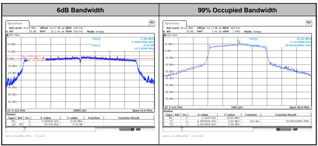
Note: The occupied channel bandwidth is maintained within the band of operation for all of the modulations.
