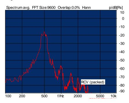
Distortion (Noise) RCV (packed): 28.58 dB (3.72%) Ok
