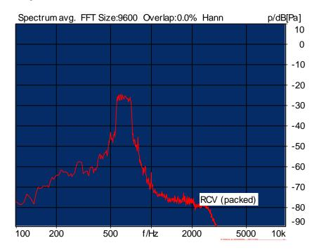
Distortion (Noise) RCV (packed): 24.45 dB (5.99%) Ok
