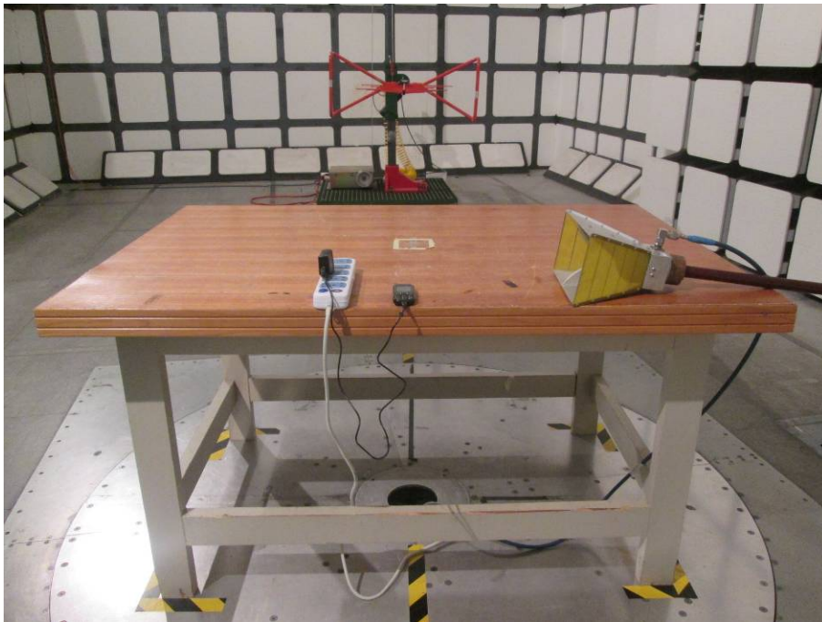
Radiated Emissions – Rear View (Below 1 GHz)
