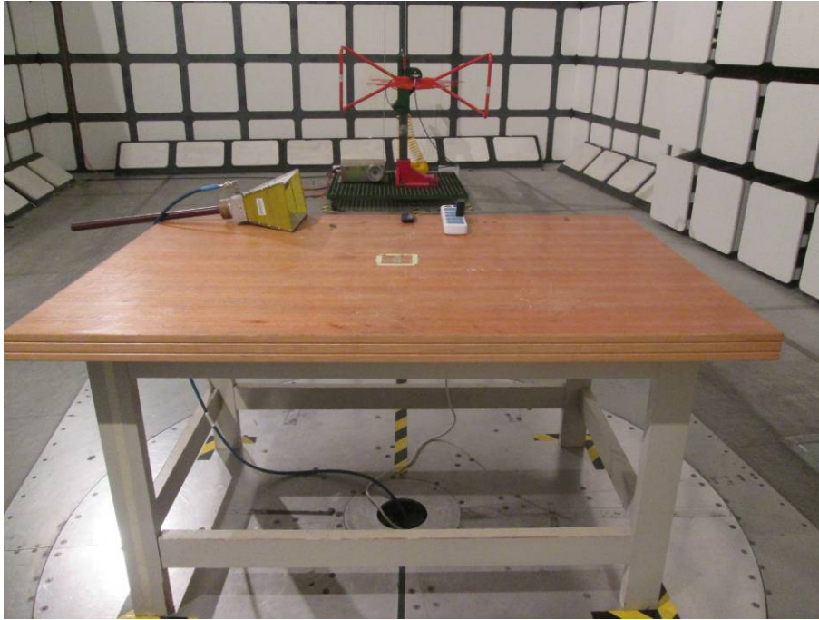
Radiated Emissions – Front View (Below 1 GHz)
