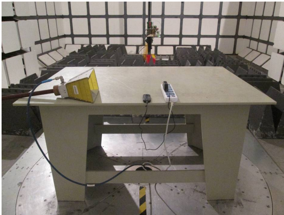
Radiated Emissions – Rear View (Above 1 GHz)
