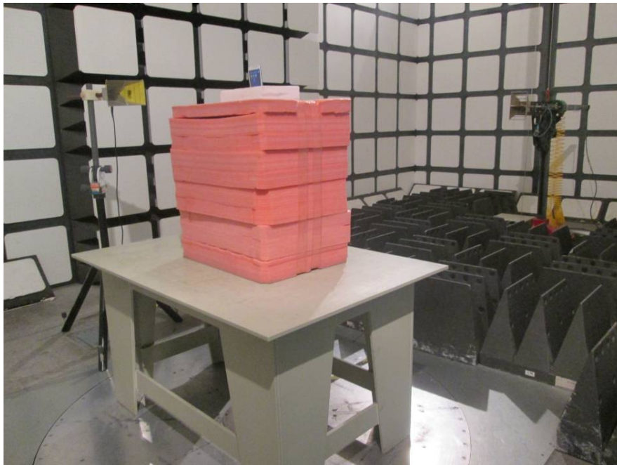
Radiated Emissions Test View (Above 1 GHz)
