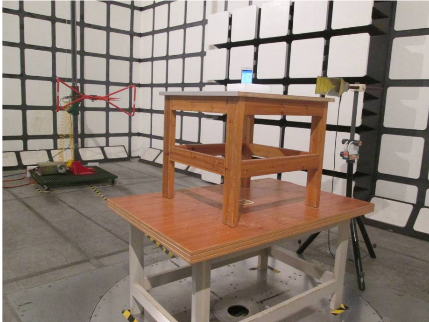
Radiated Emissions Test View (Below 1 GHz)
