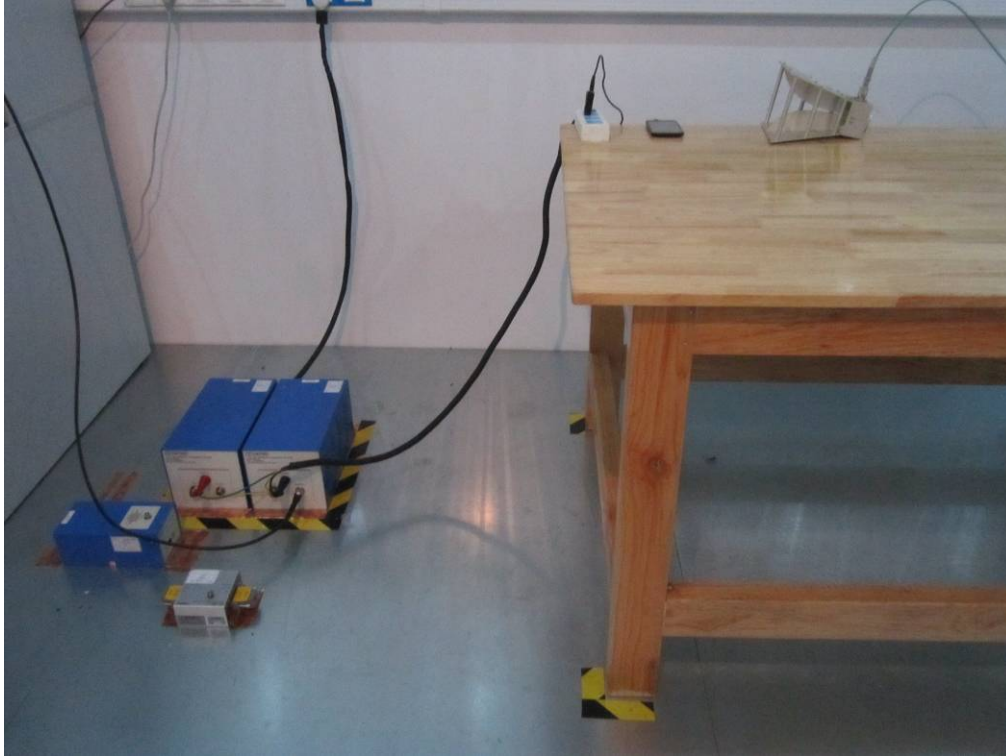
Conducted Emissions Test Setup Front View
