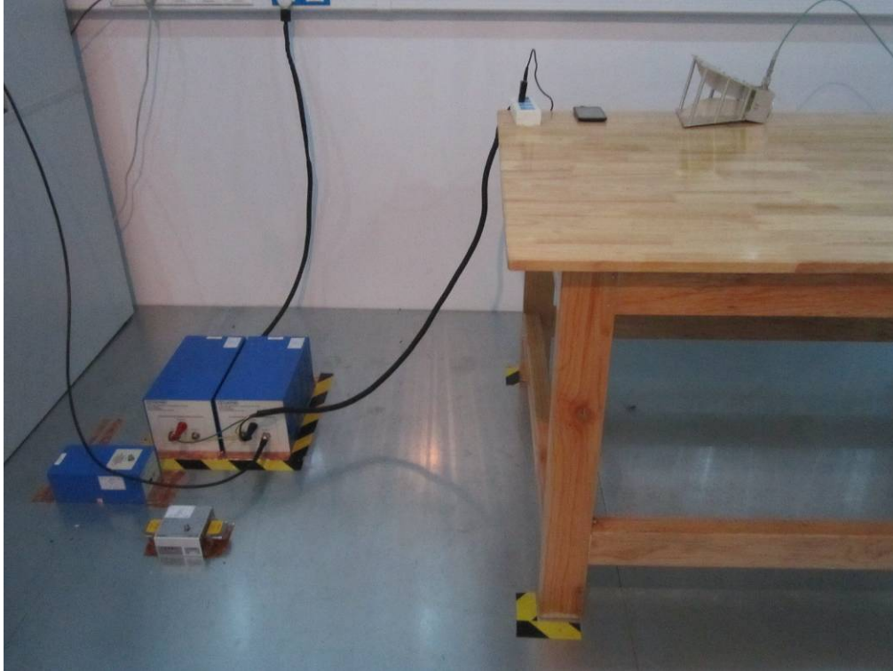
Conducted Emissions Test Setup Front View
