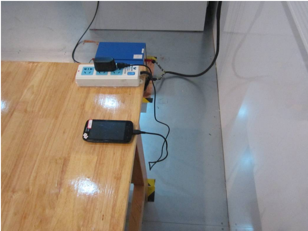
Conducted Emissions Test Setup Side View
