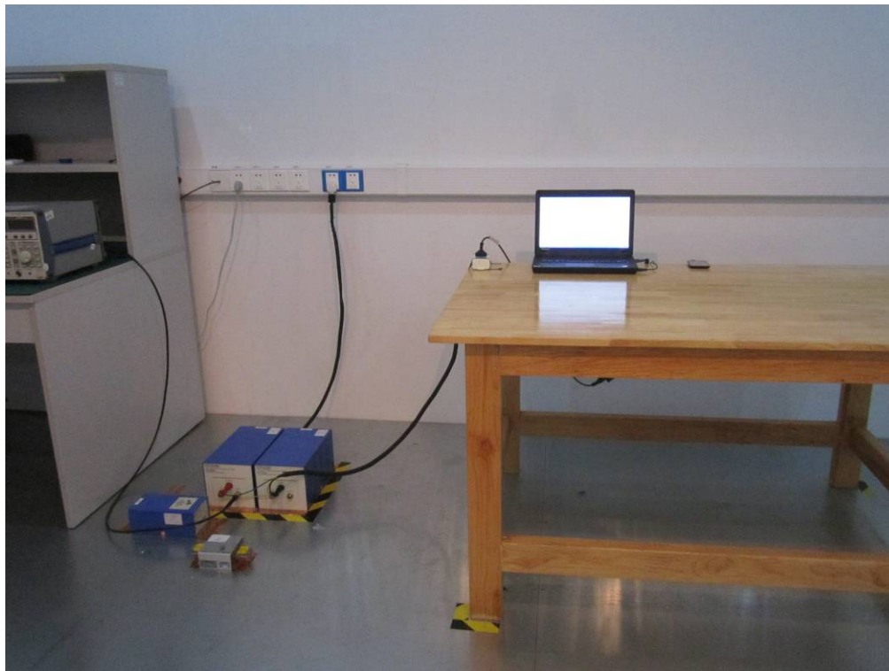
Conducted Emissions Test Setup Front View
