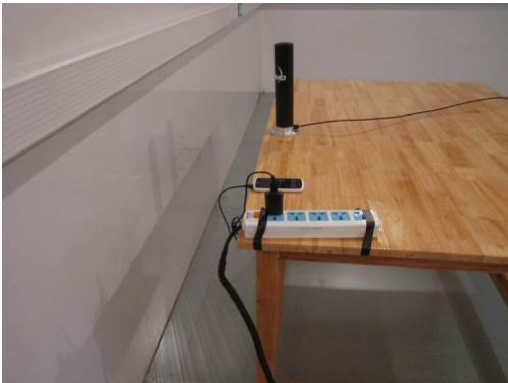
Conducted Emissions Test Setup Side View
