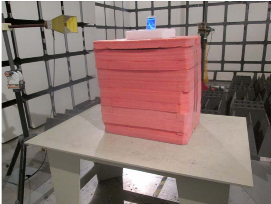
Radiated Emissions Test View (Above 1 GHz)
