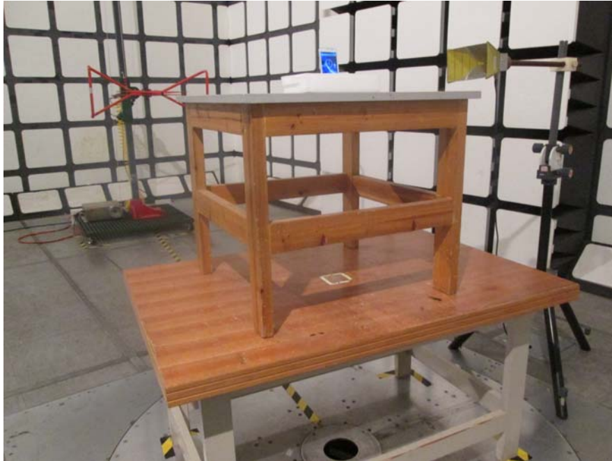
Radiated Emissions Test View (Below 1 GHz)
