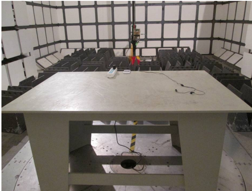
Radiated Emissions – Front View (Above 1 GHz)
