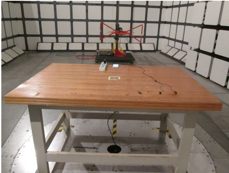
Radiated Emissions – Front View (Below 1 GHz)
