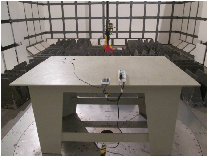
Radiated Emissions – Rear View (Above 1 GHz)
