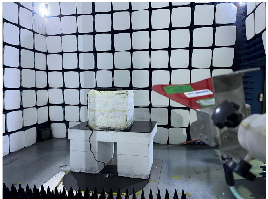
Radiation Emission Test Setup (1GHz to 18GHz)
