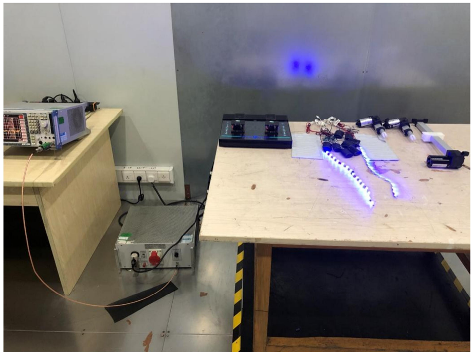
Conducted Emission Test Setup
