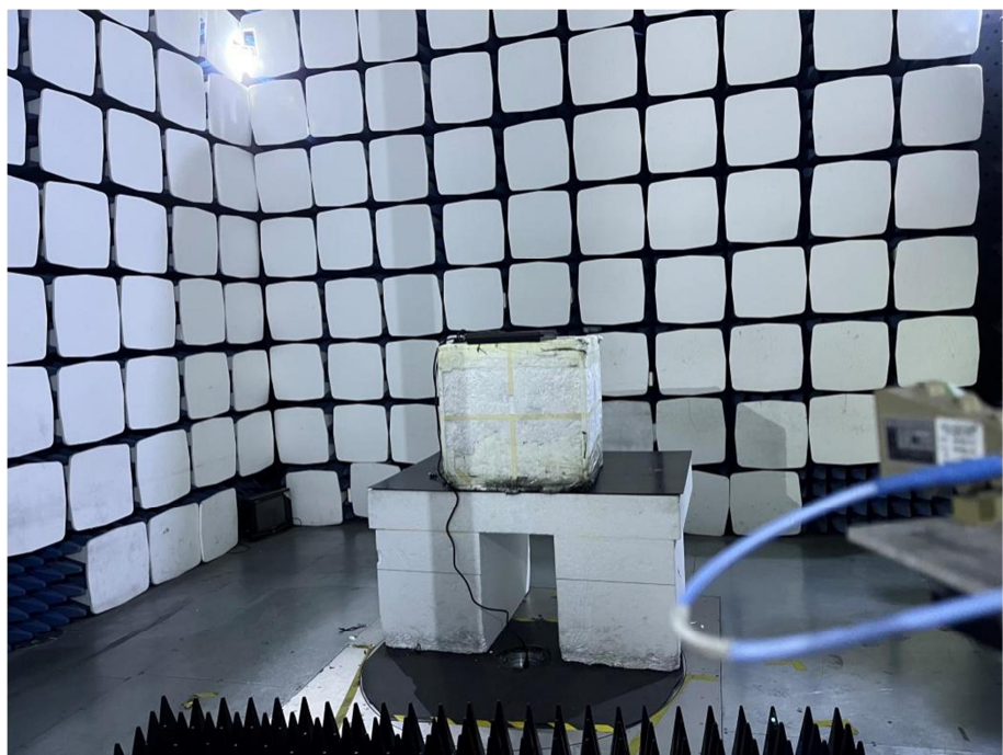
Radiation Emission Test Setup (Above 18GHz)
