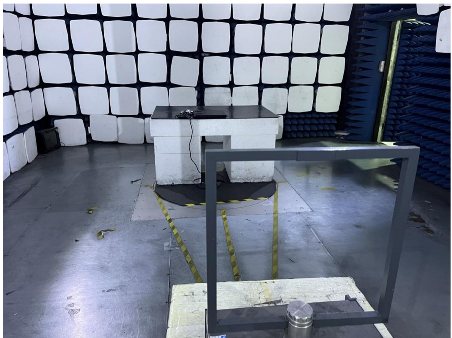
Radiation Emission Test Setup (Below 30MHz)
