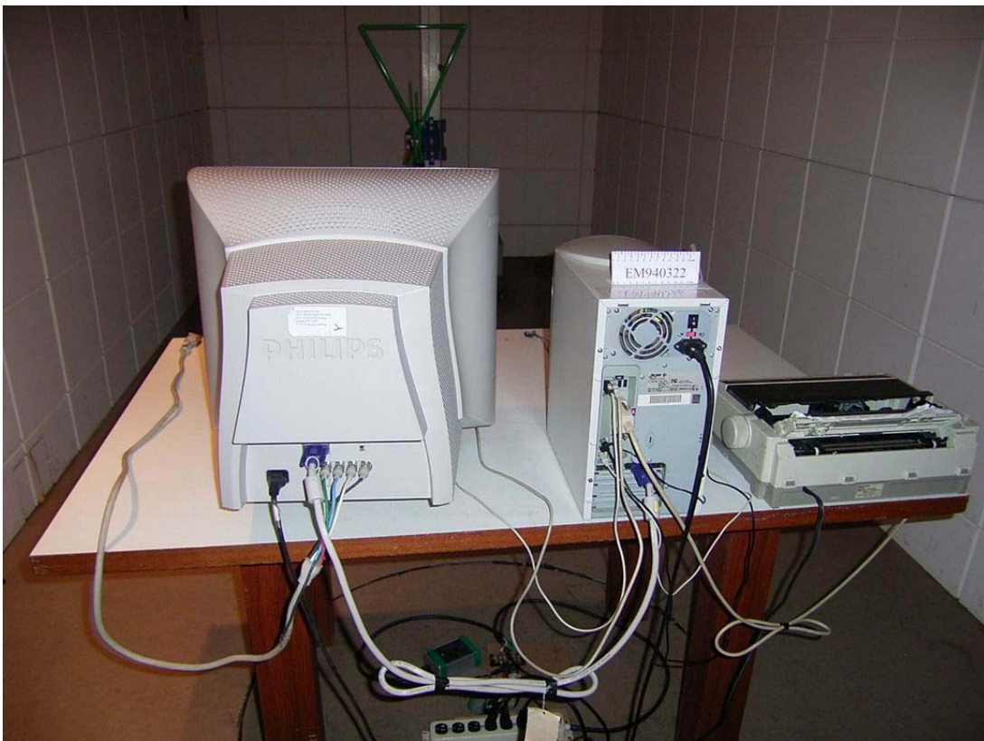
BACK VIEW OF RADIATED MEASUREMENT
