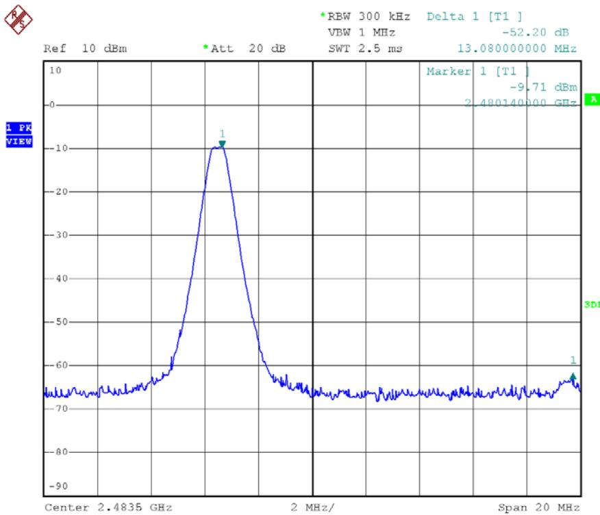
**Bandwidth / Bandedge Plot – Pursuant to FCC Part 15 Section 15. 249 Requirement (Pass/Fail)**
