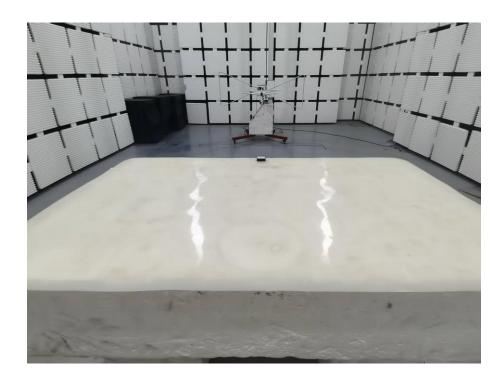
**Set-up for Radiated Spurious Emission, Above 1GHz**
