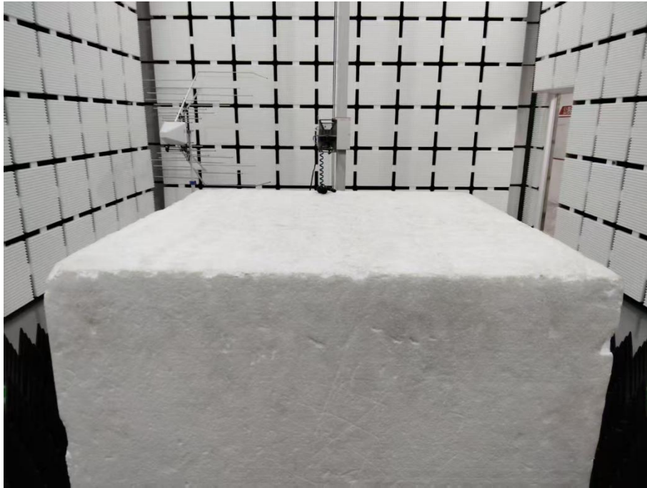
Radiated Spurious Emission (below 1GHz)
