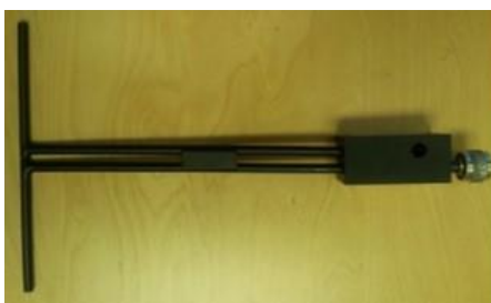
Figure 1 – MVG COMOSAR Validation Dipole
