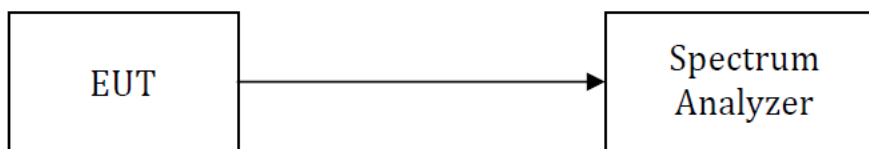
Test Setup Block Diagram
