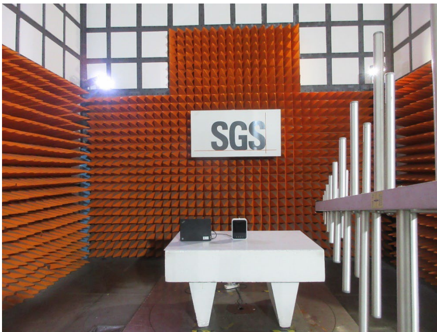
Radiated Spurious Emissions Below 1GHz
