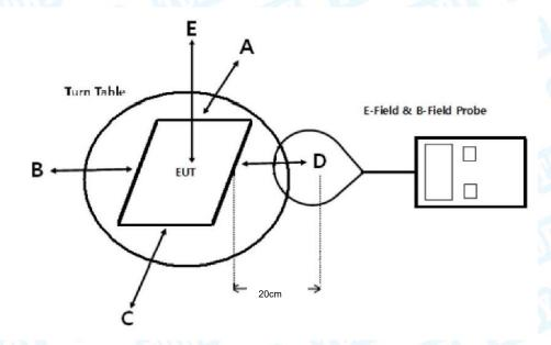
Note: The aggregate H-field strengths at 20 cm surrounding the device and 20 cm above the top surface.
