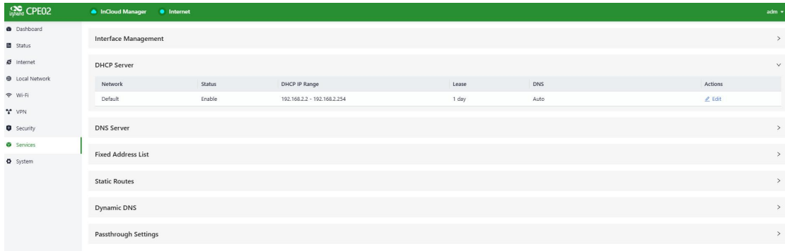
Fig. 5-8-2-a DHCP Server Panel
