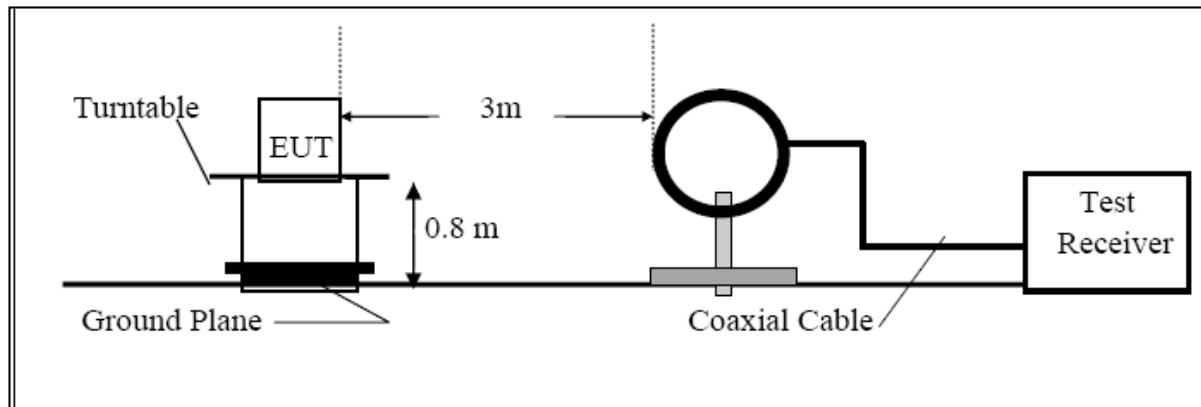
For Radiated Emission 30~1000MHz
